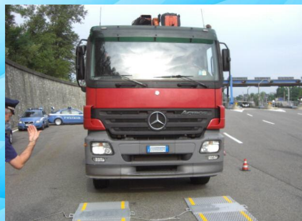
Piattaforma pesa ruote. Platform for wheels weighing.
